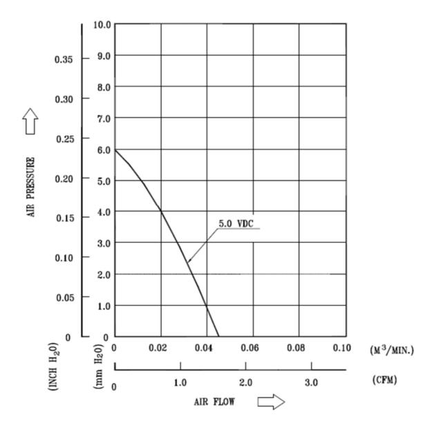
\*TEST CONDITION: INPUT VOLTAGE-----OPERATION VOLTAGE
