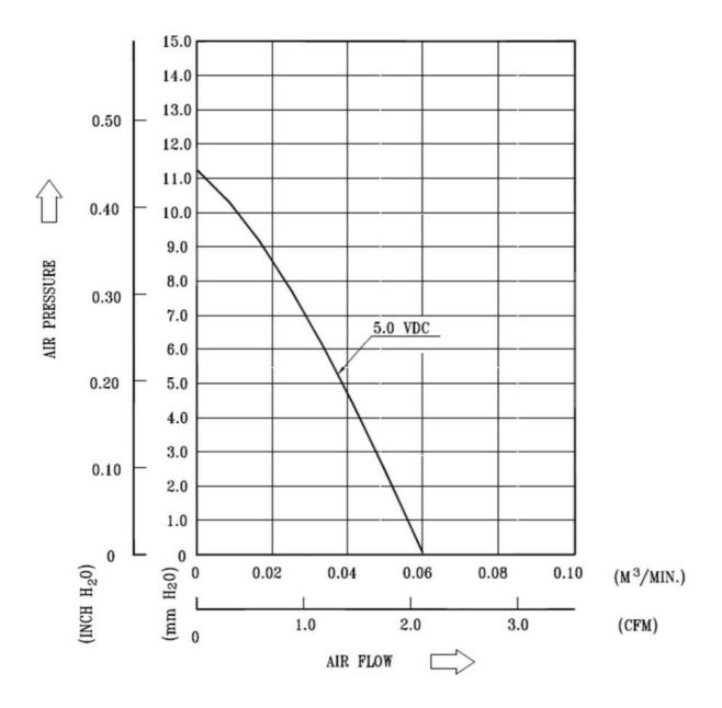
\*TEST CONDITION: INPUT VOLTAGE-----OPERATION VOLTAGE
