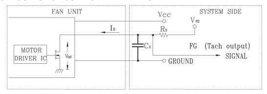
GENERAL CONDITION: VFG is 3.3V, Rx is 8.2Kohm, and Cx is 4nF. CAUTION: THE FG SIGNAL LEAD WIRE MUST BE KEPT AWAY
