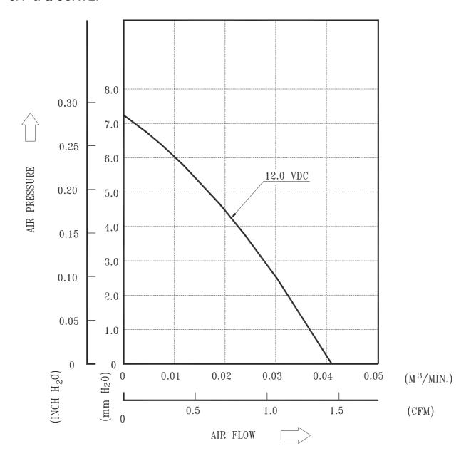
\*TEST CONDITION: INPUT VOLTAGE-----OPERATION VOLTAGE
