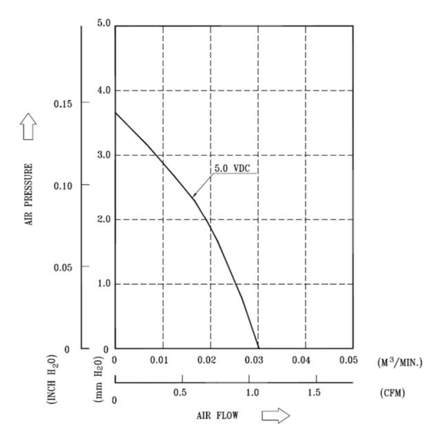
\*TEST CONDITION: INPUT VOLTAGE-----OPERATION VOLTAGE
