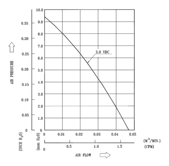
\*TEST CONDITION: INPUT VOLTAGE-----OPERATION VOLTAGE
