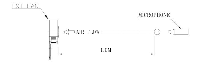
NOISE IS MEASURED AT RATED VOLTAGE IN FREE AIR IN SEMI-ANECHOIC CHAMBER WITH B & K SOUND LEVEL METER WITH MICROPHONE AT A DISTANCE OF 1.0M FROM THE FAN INTAKE.
