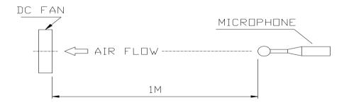
NOISE IS MEASURED AT RATED VOLTAGE IN FREE AIR IN ANECHOIC CHAMBER WITH MICROPHONE AT A DISTANCE OF ONE METER FROM THE FAN INTAKE.
