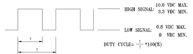
\*THE FREQUENCY FOR CONTROL SIGNAL OF THE FAN SHALL BE ABLE TO ACCEPT A 10KHZ ~ 30KHZ(REF.) WITH DIFFERENT SPEED PERFORMANCE. \*PWM SIGNAL WITH 10VDC TTL OR CMOS LEVELS. THE PREFERRED OPERATING POINT FOR THE FAN IS 20KHZ.
