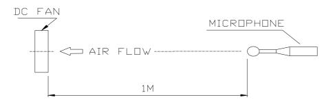
DOISE IS MEASURED AT RATED VOLTAGE IN FREE AIR IN ANECHOIC CHAMBER WITH B & K SOUND LEVEL METER WITH MICROPHONE AT A DISTANCE OF ONE METER FROM THE FAN INTAKE.
