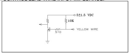
13-1. THE FAN SPEED WILL DEFAULT TO MAXIMUM WHEN THE SPEED CONTROL INPUT IS LEFT UNCONNECTED.
