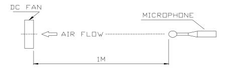
NOISE IS MEASURED AT RATED VOLTAGE IN FREE AIR IN ANECHOIC CHAMBER WITH B & K SOUND LEVEL METER WITH MICROPHONE AT A DISTANCE OF ONE METER AND 0.5 METER FROM THE FAN INTAKE.
